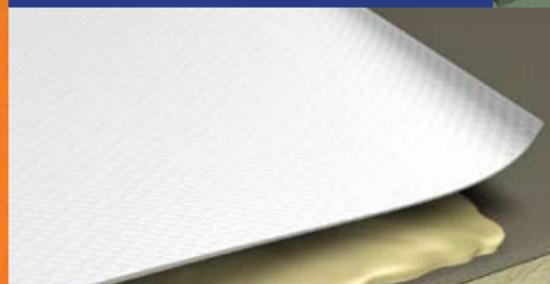
**Fully adhered** systems are ideal for roofs with unusual or odd-shaped contours, where mechanical penetration of the membrane is not desirable, yet exceptional wind performance is needed. The back of the membrane and the substrate are coated with GenFlex bonding adhesive, allowed to dry, carefully rolled back into position and broomed into place.
